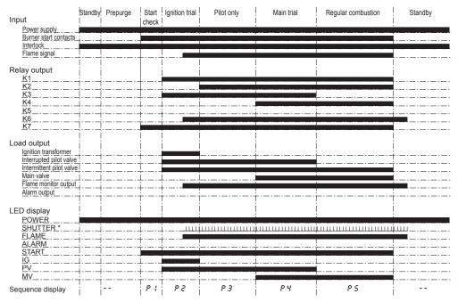
When the voltage output to the shutter is ON (opening), the shutter LED goes off. When the voltage output to the shutter is OFF (closing), the shutter LED lights up.
